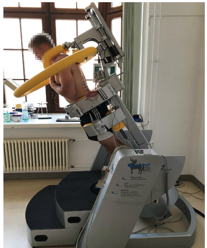
Figure 1: Subject performing the endurance task at 30° forward tilt (50% of upper body weight). Note the small feedback monitor in front of the subject for control of exact adherence to upright body posture.
