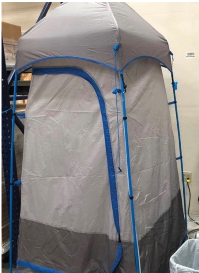
Figure 1: Replica tent for reproducing microaerosolized HOCl. The tent system used by a machine shop in another city was described to the authors and replicated within an internal laboratory. Within it was an air compressor, tubing, an HOCl reservoir, a fogging nozzle, and a chair.
