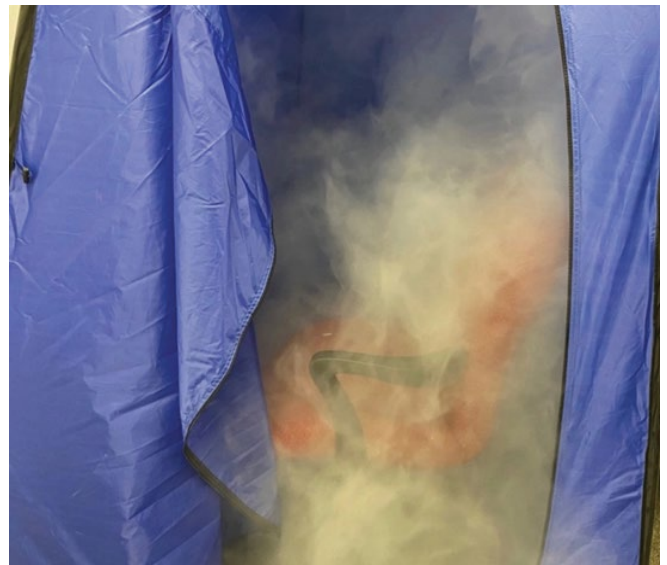
Figure 2: Tent remnants of a dense fog of microaerosolized HOCl. The fog generated by the nozzle within the tent was dense enough to obscure a hand at eye level 12 inches away. This image was taken approximately 5 seconds after opening the tent.
