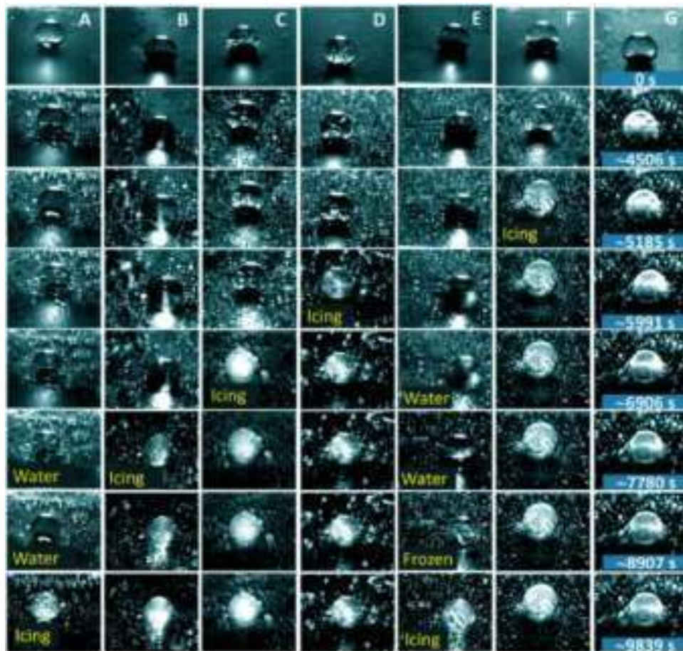
Figure 4: Microscopic images of droplets on surfaces A-G. Droplets of 7 \mu\text{L} are placed on the surface as reference [10]. The contact angle was measured on a surface of -10°C for seven different structures: A) \approx 152^\circ , B) \approx 148^\circ , C) \approx 145^\circ , D) \approx 144^\circ , E) \approx 149^\circ , F) \approx 138^\circ , and G) \approx 135^\circ . There corresponding delay times for freezing are listed in the right hand column (Figure 2).
