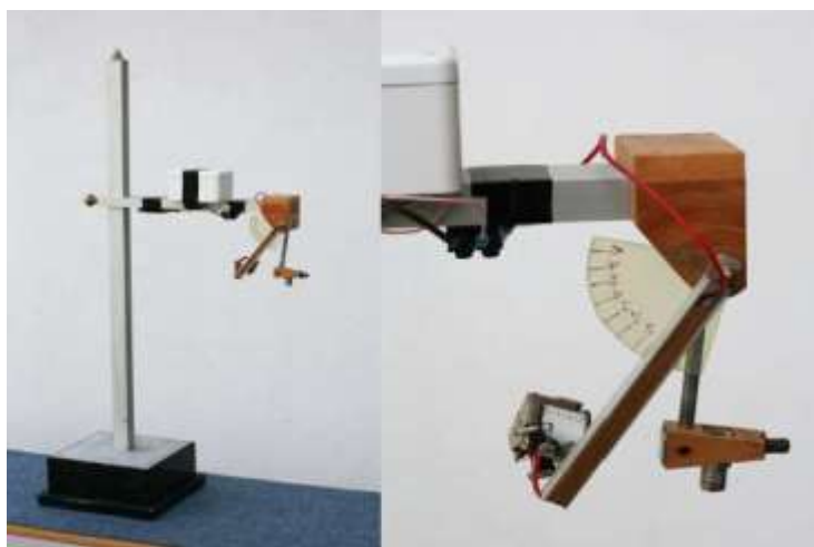
Figure 3: The support of the pendulum and the sexagesimal vernier.
