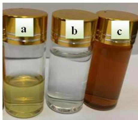
**Figure 2:** (a). Light yellow color of the reaction solution containing 1 mM  $\text{AgNO}_3$  and fungal filtrate; (b) 1 mM of  $\text{AgNO}_3$  solution; (c) Color change of the reaction solution from light yellow to dark brown indicating the formation of AgNPs.
